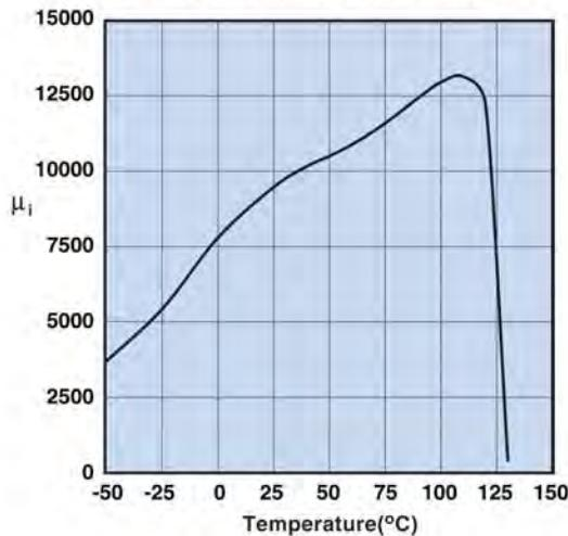
Measured on a 17/10/6mm toroid at 10 kHz.
