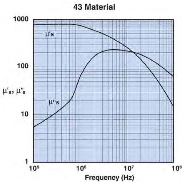
**Figure 8** Complex Permeability vs. Frequency
