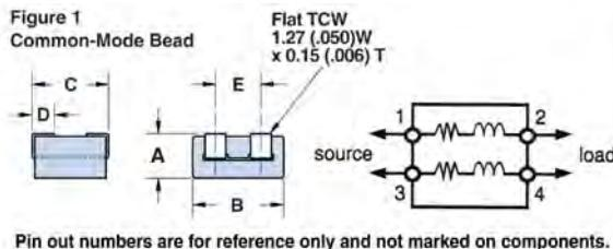
Pin out numbers are for reference only and not marked on components.
