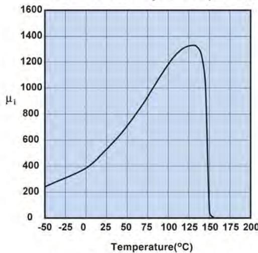
Measured on a 17/10/6mm toroid at 100 kHz.
