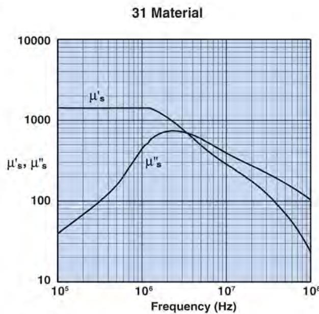
**Figure 7** Complex Permeability vs. Frequency
