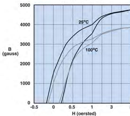
Measured on an 18/10/6mm toroid at 10 kHz.
