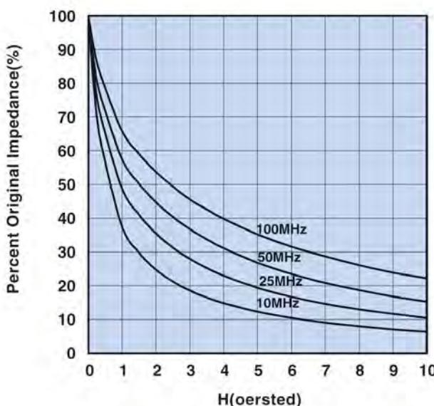
Figure 19 Percent of Original Impedance vs. Magnetic Field Strength. Measured on a 2631000301 using the HP4291A.
