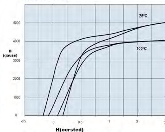
Measured on an 18/10/6mm toroid at 10kHz.
