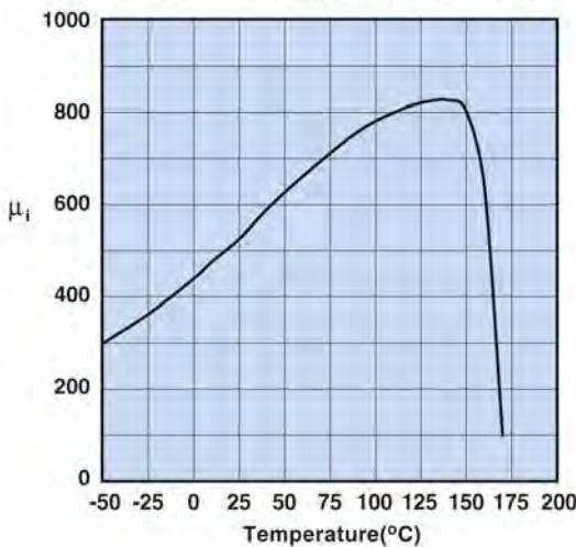
Measured on a 17/10/6mm toroid at 100 kHz.
