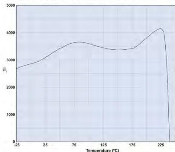
Measured on an 18/10/6mm toroid at 10kHz.
