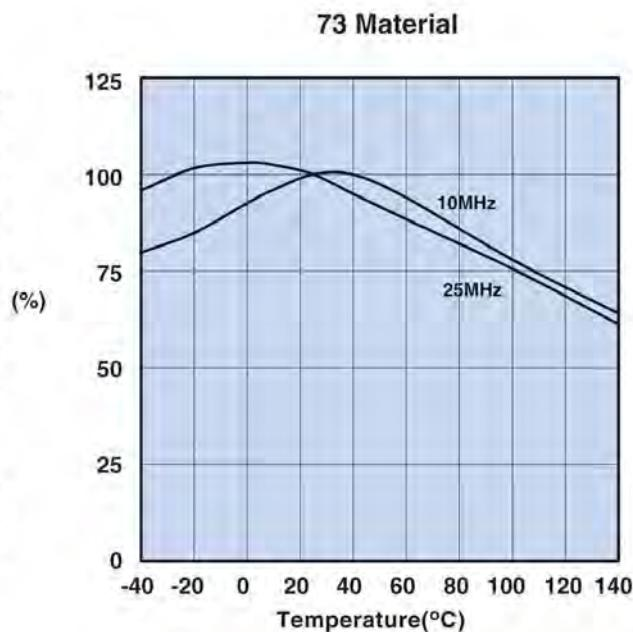
**Figure 12** Percent of Original Impedance vs. Temperature Measured on a 2673000301 using the HP4291A.
