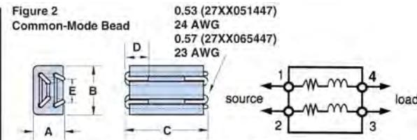
Pin out numbers are for reference only and not marked on components.
