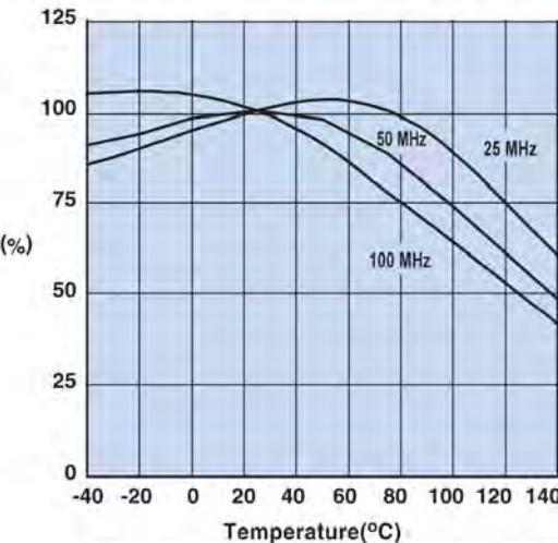
Measured on a 2646000301 using the HP4291A.
