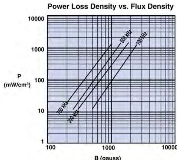
Measured on an 18/10/6mm toroid using the Clarke Hess 258 VAW at 100°C
