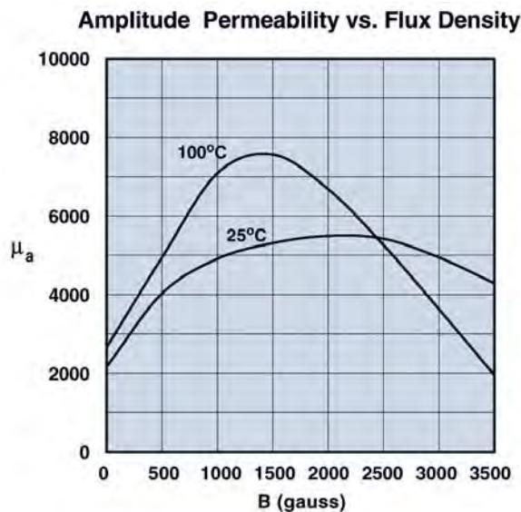
Measured on an 18/10/6mm toroid at 10 kHz.
