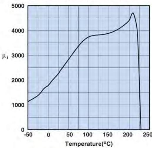
Measured on an 18/10/6mm toroid at 100 kHz.
