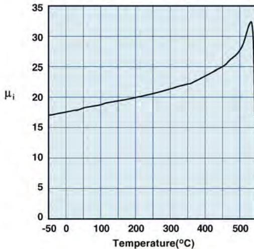
Measured on an 18/10/6mm toroid at 100 kHz.
