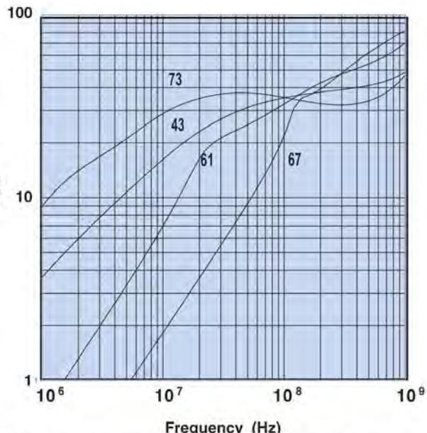
Figure 4 Impedance vs. frequency for part number 28—002302 in 73, 43, 61 & 67 material.
