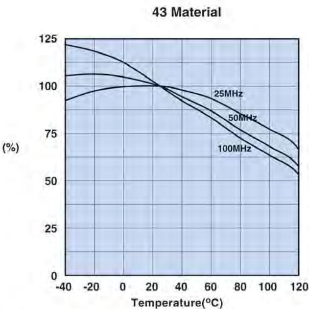
**Figure 14** Percent of Original Impedance vs. Temperature Measured on a 2643000301 using the HP4291A.
