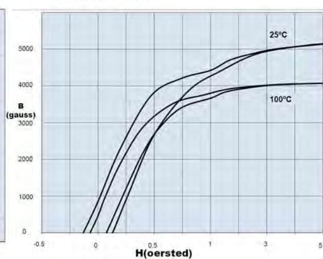
Measured on an 18/10/6mm toroid at 10kHz.
