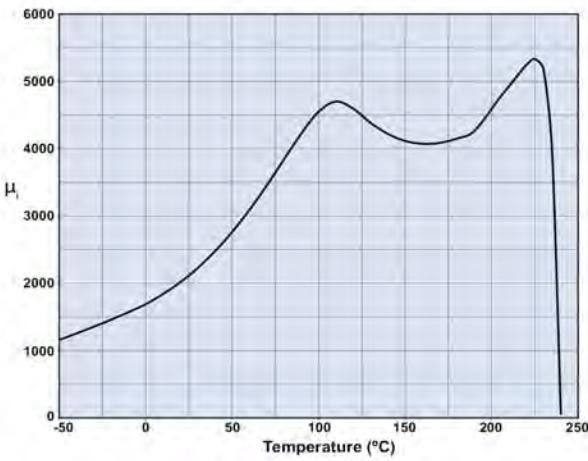
Measured on an 18/10/6mm toroid at 10kHz.
