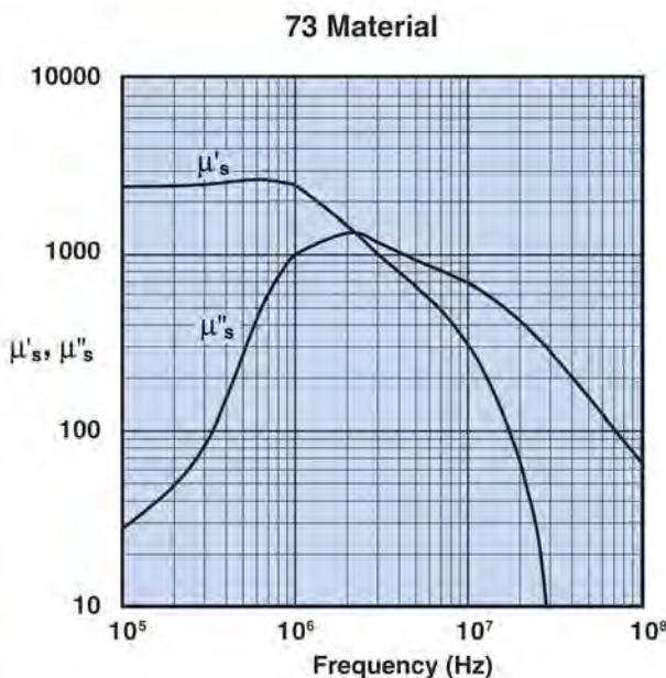
**Figure 6** Complex Permeability vs. Frequency
