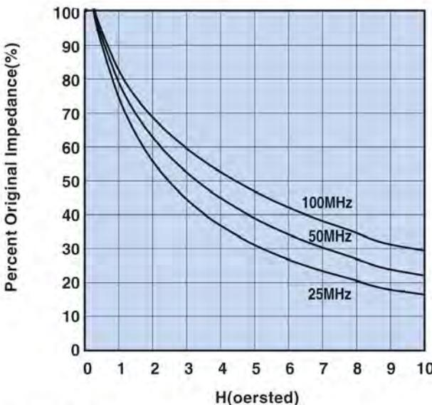
Figure 21 Percent of Original Impedance vs. Magnetic Field Strength. Measured on a 2644000301 using the HP4291A.
