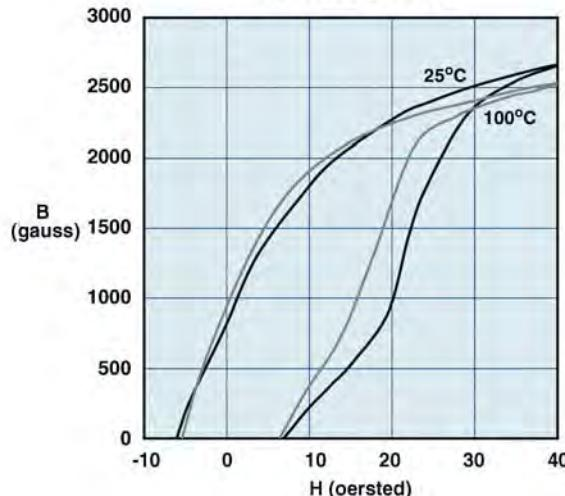
Measured on an 18/10/6mm toroid at 10 kHz.
