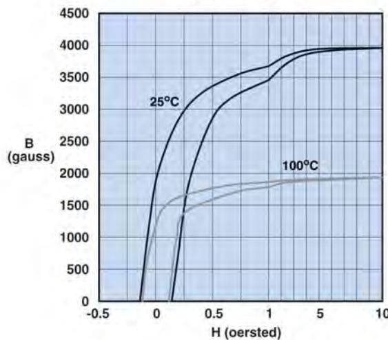
Measured on a 17/10/6mm toroid at 10 kHz.
