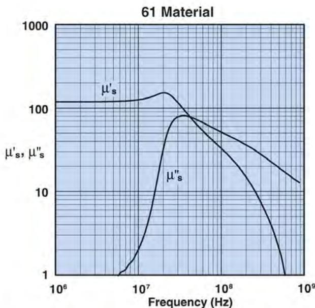
**Figure 11** Complex Permeability vs. Frequency
