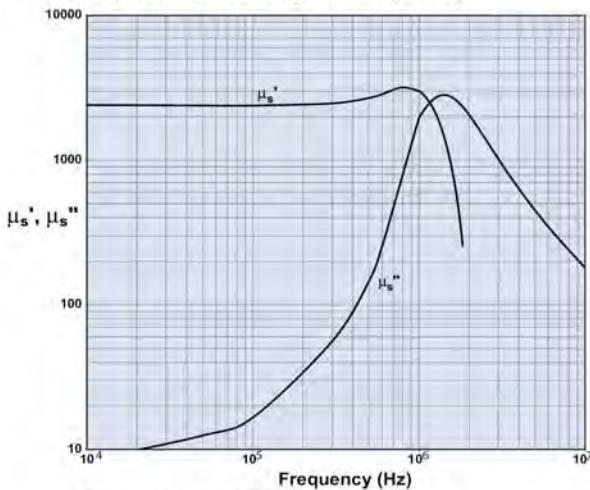
Measured on an 18/10/6mm toroid using HP 4284A and HP4291A.
