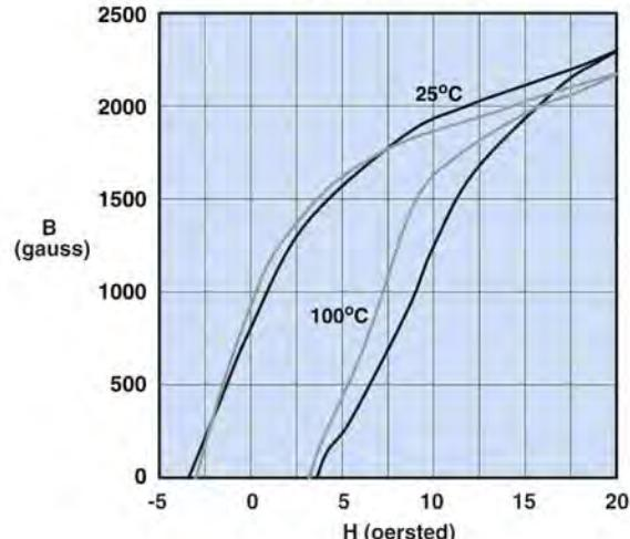
Measured on a 19/10/6mm toroid at 10 kHz.
