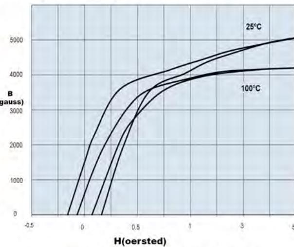
Measured on an 18/10/6mm toroid at 10kHz.
