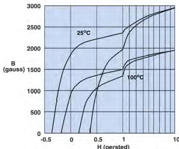
Measured on a 17/10/6mm toroid at 10 kHz.
