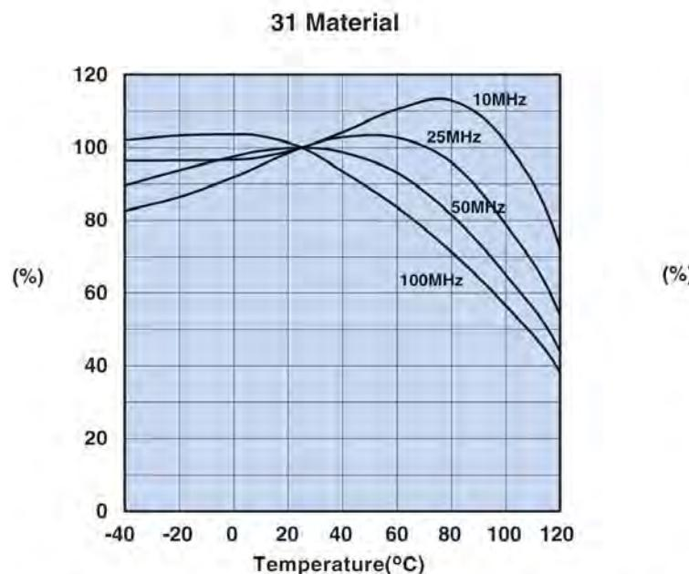
**Figure 13** Percent of Original Impedance vs. Temperature Measured on a 2631000301 using the HP4291A.
