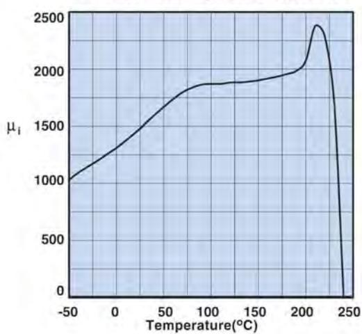
Measured on an 18/10/6mm toroid at 100 kHz.
