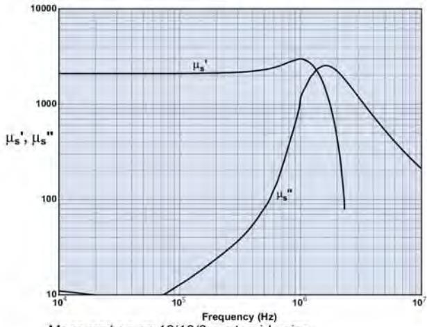
Measured on an 18/10/6mm toroid using
