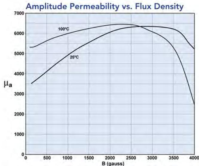
Measured on an 18/10/6mm toroid at 10kHz.
