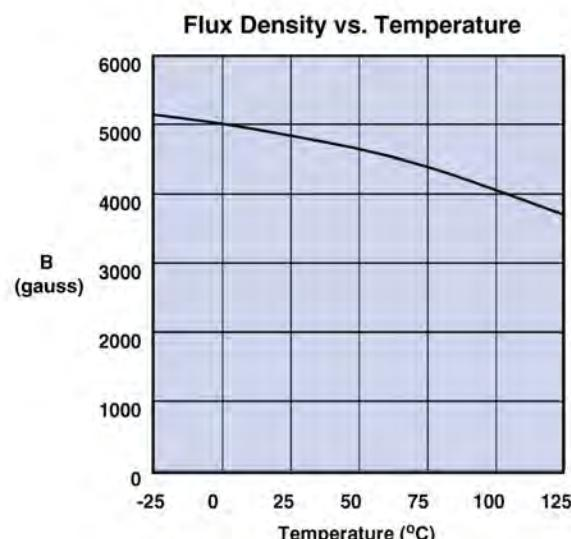
Measured on an 18/10/6mm toroid at 10 kHz. and H=5 oersted.
