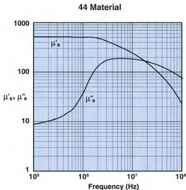
**Figure 9** Complex Permeability vs. Frequency
