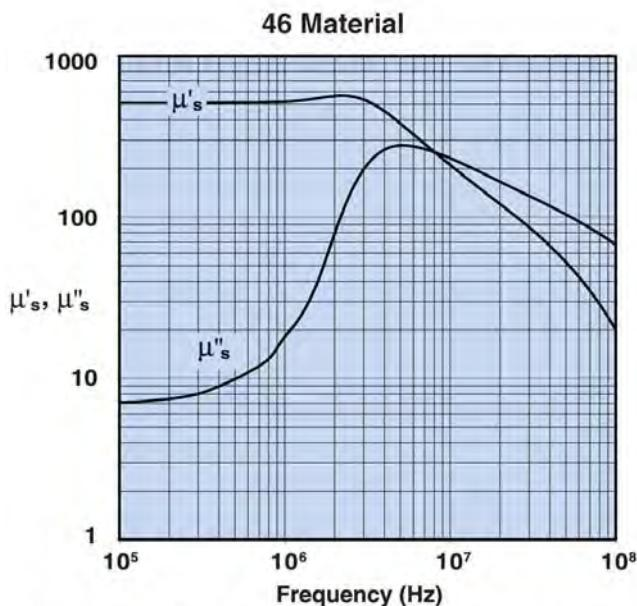
**Figure 10** Complex Permeability vs. Frequency
